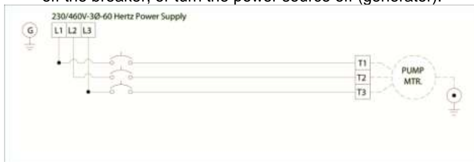
Typical 3 phase manual control 1
