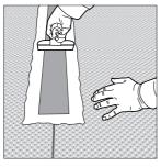
3. To waterproof around the walls of the installation area, take a pre-measured length of USG Durock™ Waterproofing Membrane Band and fold it in half along its length. One side of the fold will be adhered to the floor and the other side will be adhered up the wall. Follow the first two steps for applying mortar and embedding USG Durock™ Waterproofing Membrane Band.
