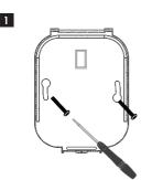
Insert fixing screws through mounting holes of the power base and tighten.
