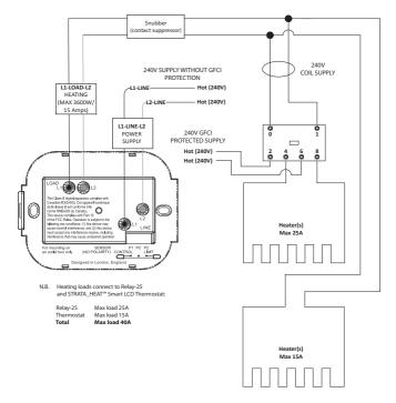
Heating Load connected to Relay 25 - Max. 25 Amps
