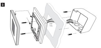
Install a 3–1/2" (89 mm) deep single gang or 2–gang box with mud ring in your preferred thermostat location. Pull wires (heater, supply and sensor) through gang box and complete terminal wiring.
