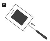
Unclip the display from the power base and remove the display
