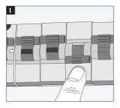
Isolate the STRATA\_HEAT Smart LCD Thermostat and supply from the mains supply.
