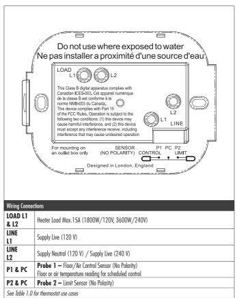
NOTE: The function of Probe 1, Probe 2 from Control/Limit Sensor can be swapped in Advanced Settings; Sensors & Application.
