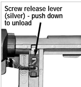
Screw release lever (silver) - push down to unload
