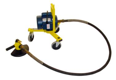
Northrock's line of hand-held grinders are perfect for finishing terrazzo or other concrete applications. They are ideal for grinding, trimming, sanding, and buffing.
