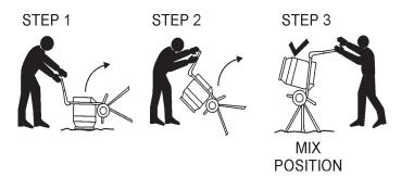
**Figure 14. Tilting Mixer to Upright Position**
