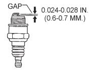
Figure 32. Spark Plug Gap
