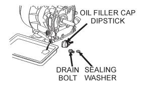
Figure 33. Engine Oil (Draining)
