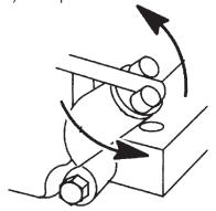
Figure 15. Engine Oil Dipstick (Removal)
