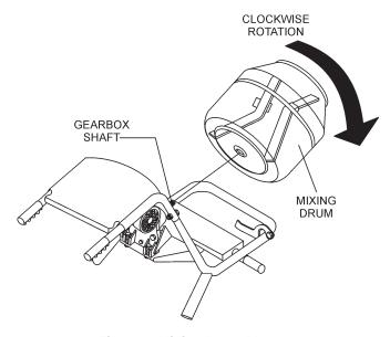
**Figure 8. Mixing Drum Placement**
