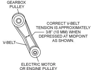
Figure 31. V-belt Adjustment
