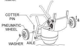
Figure 11. Wheels and Wheel Retainers
