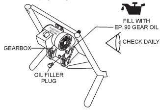
Figure 30. Gearbox Oil Level Check
