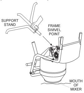
Figure 10. Attaching Support Stand
