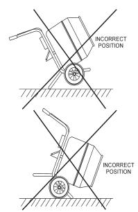
Figure 29. Mixer Positioning (Gearbox Oil Level)
