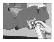
(E) Lubricate the Blade Shaft
