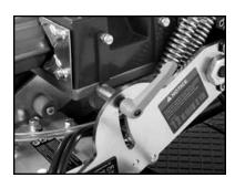
(D) Loosen the Cutting Head Height Lock.
