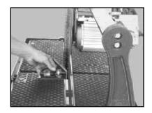
(C) Check the Cutting Head alignment.
