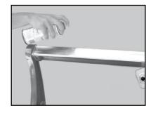
(C) Lubricate the Guide Rail.
