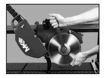
(F) Reinstall the Inner Flange and Blade.
