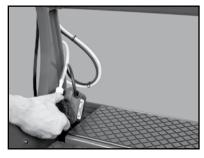
(A) Remove water pump from water pan.
