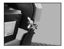
(F) Loosen the Blade Guard Pivot Point Retaining Wingnut.
