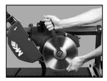
(O) Tighten the Blade Retaining Nut.
