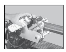
(E) Lubricate the Cutting Head springs.
