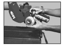
(C) Lubricate the Inner Flange Gasket.
