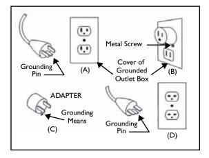
Fig. 1 Circuit and Adapter Information
