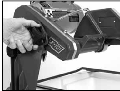
(E) Install the Adjusting Knob
