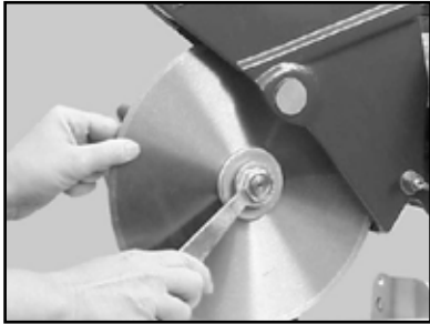
(A) Remove the Diamond Blade
