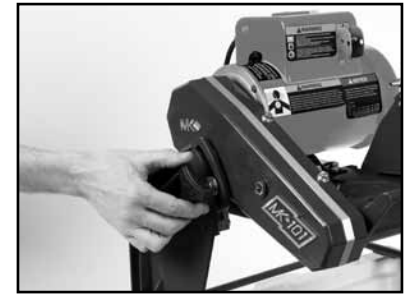
(C) Ensure the Adjusting Knob is tight
