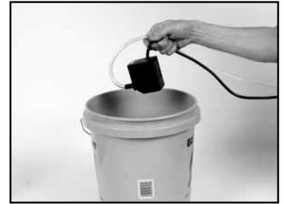
(C) Place Pump into a bucket of water and check flow
