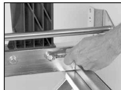
(C) Loosen the Retaining Bolts.
