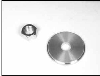
(B) Lubricate the Outer Flange and Retaining-nut
