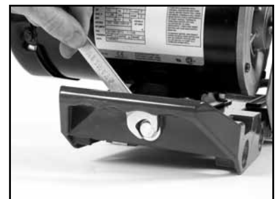
(I) Loosen the Motor Adjustment Strap
