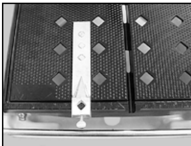
(B) Position the Adjustable Cutting Guide to desired cut length
