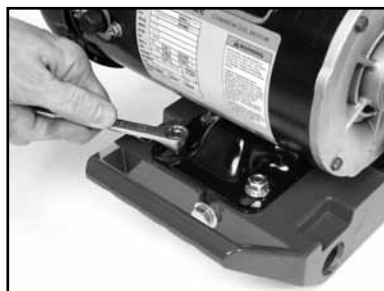
(H) Loosen the two back motor mounting bolts
