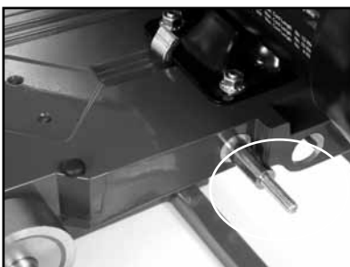
(G) Lubricate the Blade Guard Pivot Shaft
