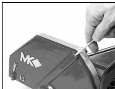
(H) Rod Cooling Channels and recheck flow
