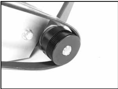
(M) Verify the Micro-V Belt is seated in the grooves of both pulleys
