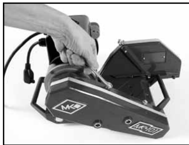
(Q) Install the Belt Guard
