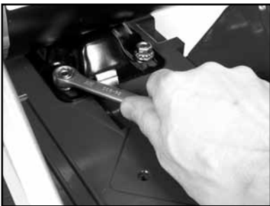
(P) Tighten the four motor mounting bolts
