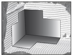
Continue with thin-set along the floor-to-wall transition from the corner outward for the first strip of HYDRO BAN Sheet Membrane Sealing Tape. Overlap the corners by 2" (50 mm).
