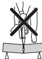
If the blade is pinched or stalled in the kickback zone, the reactive force will push the power cutter up and back towards the user in a rotating motion causing serious or even fatal injury. Be alert for potential movement of the work piece. If the work piece is not properly supported and shifts as you cut, it might pinch the blade and cause a kick back.
