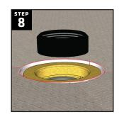
Slide the rubber caulking gasket (bevel side up) over the 2" drain pipe until it is flush with the top of your drain pipe. Ensure that the rubber gasket is not higher than the top of the 2" drain pipe. Soapy water may be used to help ease the rubber gasket onto the pipe. DO NOT use a petroleum based lubricant.
