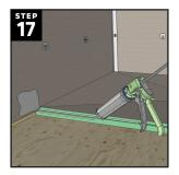
Begin installing the HYDRO-BLOK Shower Curb by cutting the shower curb 1/8" shorter than the distance between the two shower walls where the curb will be placed. If your shower requires curbs on two sides of the shower pan see the Installation Tips on the back page of this guide.
