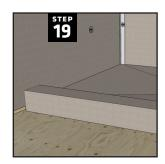
Position the shower curb ensuring the curb is firmly pressed into place against the shower pan notch and the thinset on the sub floor.
