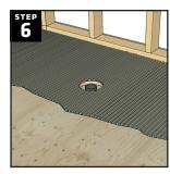
Mix modifed thinset as per manufacturer's instructions. Apply thinset to the subfloor starting at the back of the shower area, troweling towards the front. Ensure the trowel lines are pointing to the front or curb of your shower pan. This will ensure there will be no voids in the installation. DO NOT cross channel trowel lines or air can not escape.
