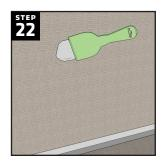
Perform a final check of all joints and screws/washers to ensure they are completely covered in joint sealant. Check the caulking nut on the drain assembly again to ensure it is tight and cannot be turned by hand with a screwdriver.
