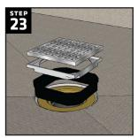
Loosely fit the HYDRO-BLOK stainless steel drain and tray into the shower pan drain opening while installing tile (tile up to the edge of the tray).
