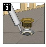
Apply a continuous ¼" bead of HYDRO-BLOK Joint Sealant around the top edge of the first notch inside the shower drain profile ensuring that the bead is consistent and full. Drop the solid brass drain body into the joint sealant and seat it firmly.
