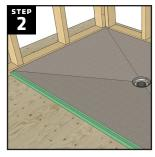
Dry fit the shower pan on the subfloor and ensure that the subfloor opening and drain pipe are centered inside your shower pan drain opening. Ensure all sides of the shower pan fit comfortably to the walls. DO NOT try to force the shower pan into its location.
