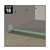
Trowel thinset out from the shower pan edge to the edge of the curb location. Trowel away from the pan in one direction. Apply thinset on the underside of the shower curb with the smooth edge of the trowel. Ensure the thinset does not contact or mix with the joint sealant, cleaning off any excess thinset from the joints of the shower curb.
