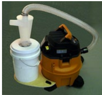
Bolt to Attached Platform - This works best with large wet / dry vacuum.
