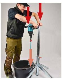
For mixing: push the machine into the material and move to all sides.
