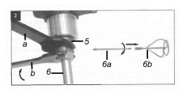
First screw mixer shaft (6a) together with mixer paddle (6b). Screw the mixer paddle (6) into the mixer (5). Use the two wrenches to tighten. Use one of the wrenches (a) to hold the mixer (5) in place and then use the second wrench (b) to tighten up the mixer (6). Proceed in the reverse sequence to undo the paddle from the mixer.
