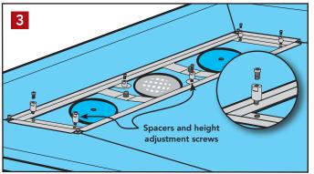
You can install the cover so it's on display, or flip it over and fill it with tile or stone. If you intend to show the steel, install spacers and height adjustment screws ( $\gamma_{16}$ " long) in the six locations shown. If you plan to fill the cover, install only the height adjustment screws (no spacers).
