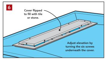
If you prefer to fill the cover, first rough-up its inside surfaces with 80 grit sandpaper, then clean them with a damp cloth. After it's completely dry, brush a coat of Tank/ $10^{\circ}$  waterproofing onto the steel (to improve mortar adhesion). Use a modified thinset mortar to bed your tile or stone.
