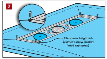
Insert a tile spacer height adjustment bolt into the threaded hole located at each corner of the tile adaptor. Identify these four bolts by their overall length: a bit over ¾" (the longer bolts in the hardware kit). Turn the bolts until the heads contact the tile adaptor (use a hex driver if necessary).
