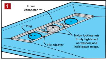
Place the tiling adaptor into the drain gulley so that the hole in each holddown strap slips onto a threaded stud in the gulley. Slip a washer onto each stud and follow with a nylon locking nut. Tighten the nuts firmly to secure the tile adaptor to the gulley floor.
