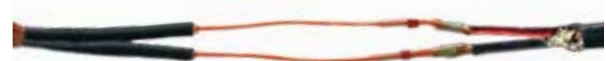
Fig. 3.31: Push the heat-shrink tubing further back and cover with damp cloth before soldering tubes.
