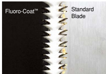
*After cutting through 40 mm thick branches, 100 times.
