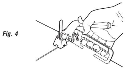
*Important note:* When inserting the caps and strap under the side of the tile, DO NOT place them at the tile corners. Inserting them on tile corners will prevent an accurate installation, and could crack or break the corners of the tiles when removed. It will also be very hard to keep the grout joint line straight.
