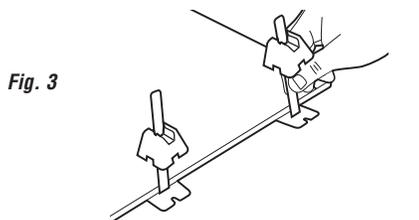
To facilitate a speedy installation, pre-assemble the straps and caps you will need for the days work, leaving 1-1/2 to 2 in. between the bottom of the caps and the strap bottom plate. See Fig. 2.
