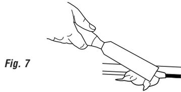
On the following day, begin by making sure you fill the hollow spots from the previous day with a margin trowel and ‘pack’ the tile underneath with thinset. Insert the straps and caps and start your installation again, following the same process as before. See Fig. 7.
