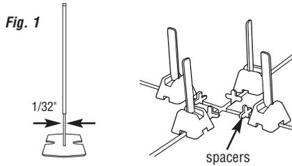
The Tuscan Leveling System™ straps will achieve a 1/32 in. grout joint, if you want a wider joint, you can use the Tuscan Leveling System™ with most common spacers. Simply insert corner or side spacers of the desired width, up to 1/2 in. See Fig. 1.
