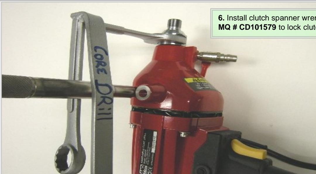
6. Install clutch spanner wrench MQ # CD101579 to lock clutch.
