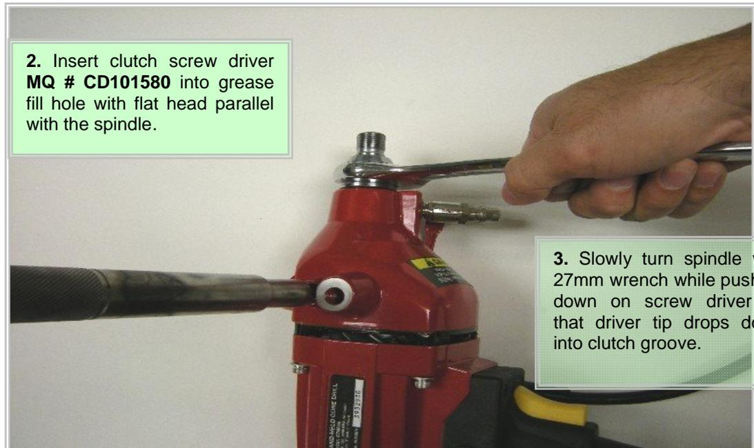
4. Once the tool is engaged tighten the clutch by turning the spindle with wrench in the direction of the arrow.
