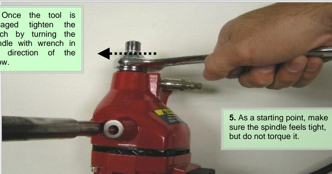
5. As a starting point, make sure the spindle feels tight, but do not torque it.
