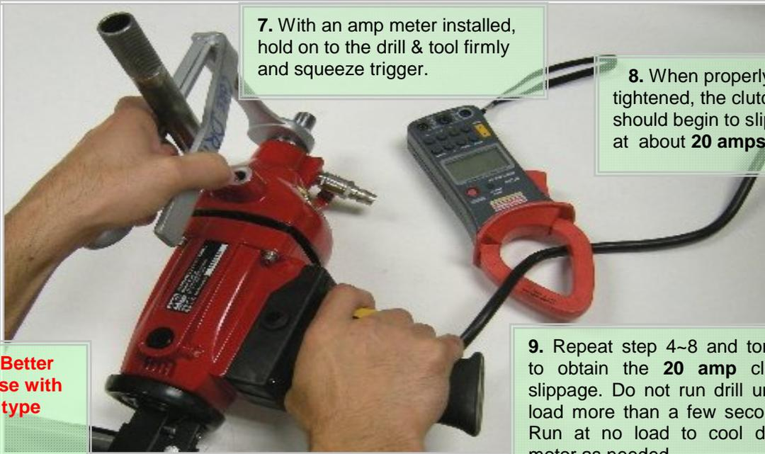
7. With an amp meter installed, hold on to the drill & tool firmly and squeeze trigger.
