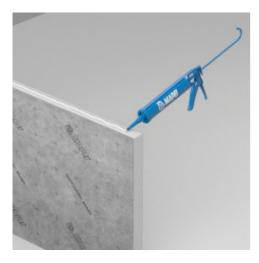
• Mapeguard Board has a waterproof surface: to guarantee the <u>waterproofing</u> of the wall or assembled element, it is sufficient to seal the joints between each single panel with Mapeguard ST tape and all the critical areas (corners, edges, through elements) with the special accessory items from the Mapeguard system (Mapeguard IC, Mapeguard EC, Mapeguard PC). Mapeguard accessory items can be applied using Mapeguard WP Adhesive.
