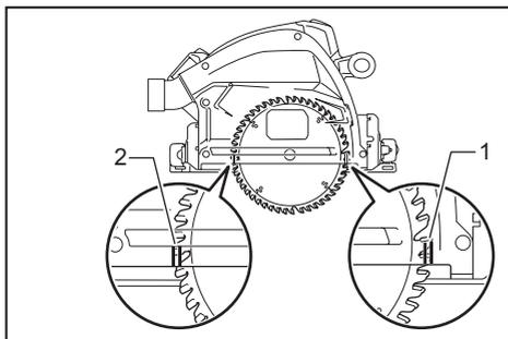
► 1. Front cutting point 2. Rear cutting point
