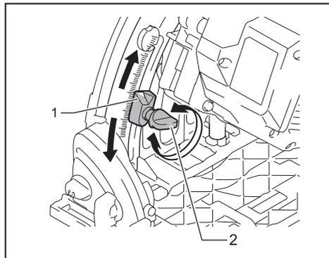
► 1. Blade lower limit stopper 2. Clamping screw
