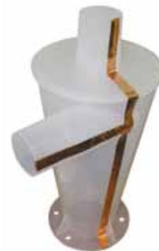
Cover bolt hole and use the bolt for the grounding wire anchor.
