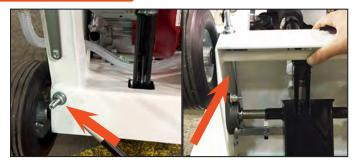
Revised tensioning system to the motor gives direct tension to the belts for better distribution of power providing more horsepower.
