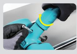
3.2 Loose the handle and put in the cutting wheel then fasten the handle, choose 4 for cutting 4mm tiles, choose 10 for cutting 10mm tiles etc.. **3.3** Fix the Straight and Swiveling Guide with two bolts and adjust the side ruler to the required angle
